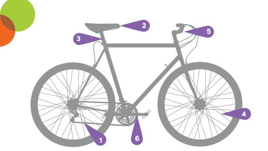
5. Handlebars 6. Crank 1. Chain 2. Saddle 3. Seatpost 4. Spoke
